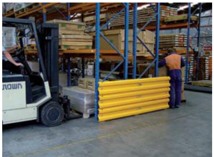
Three high barrier protecting the end of pallet racking.
