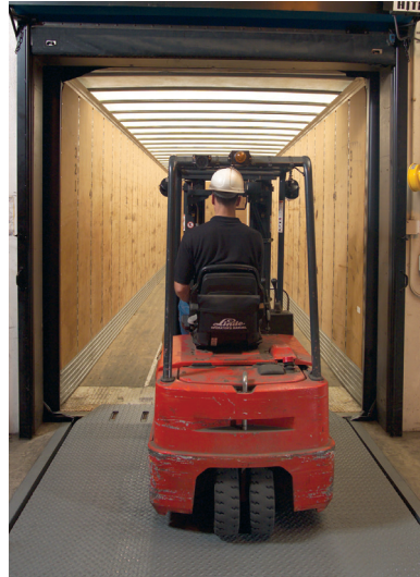
Gaps are sealed by GapMaster hooks, without restricting access to the trailer.
