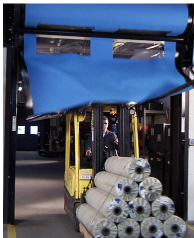
As it's raised, the FasTrax door curtain automatically re-feeds itself back into the side frames.
