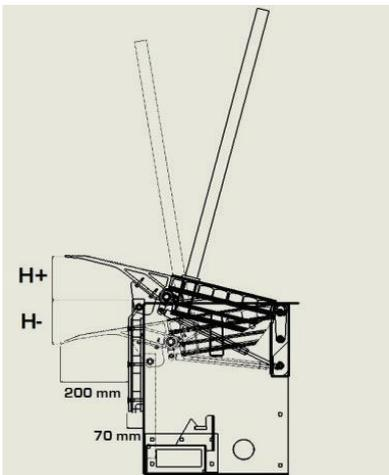
Optional: OVERBAY INSTALLATION STRUCTURE the structure is to be welded to a U profile already put into the loading bay border during concrete cast
